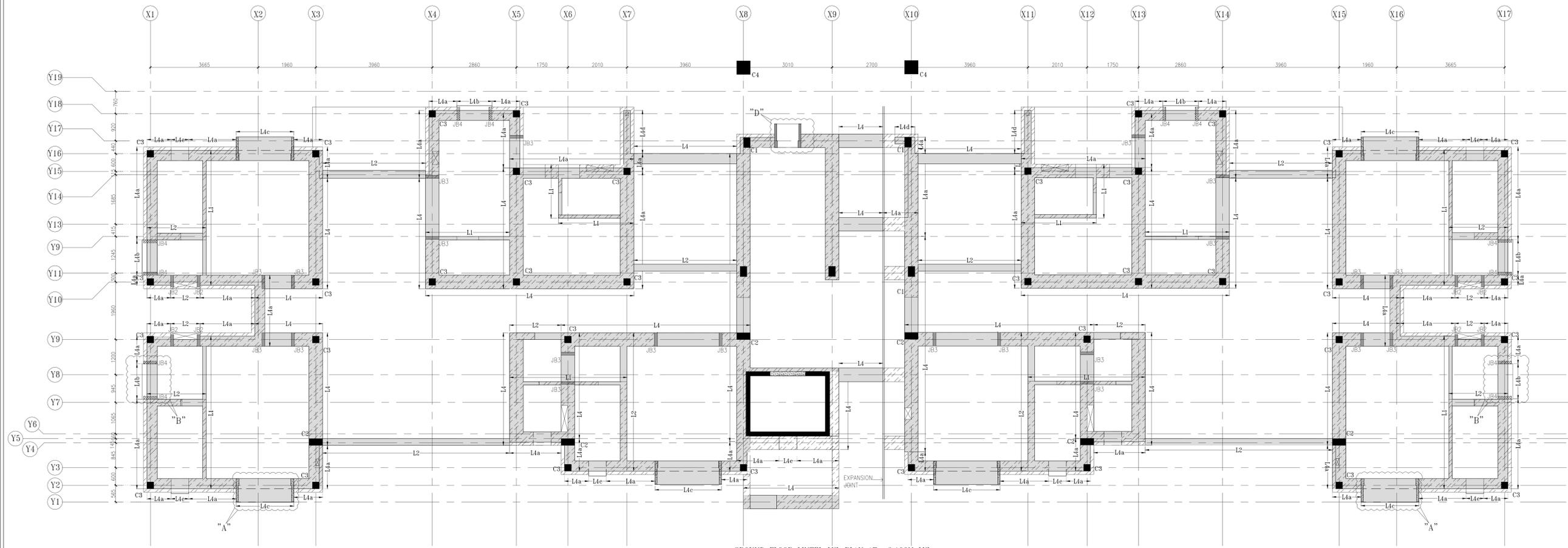
GROUND FLOOR LINTEL LVL PLAN AT +2.100M LVL.
