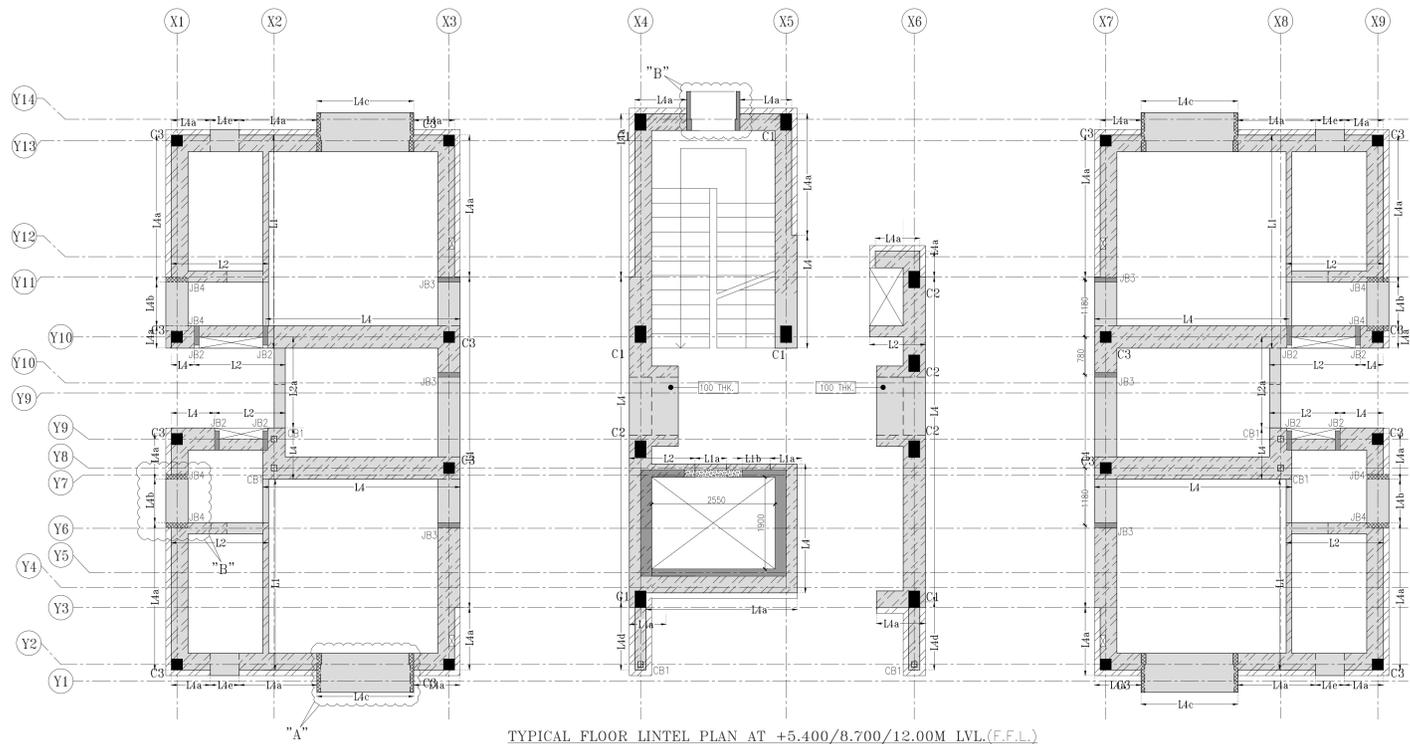
TYPICAL FLOOR LINTEL PLAN AT +5.400/8.700/12.00M LVL (F.F.L.)
