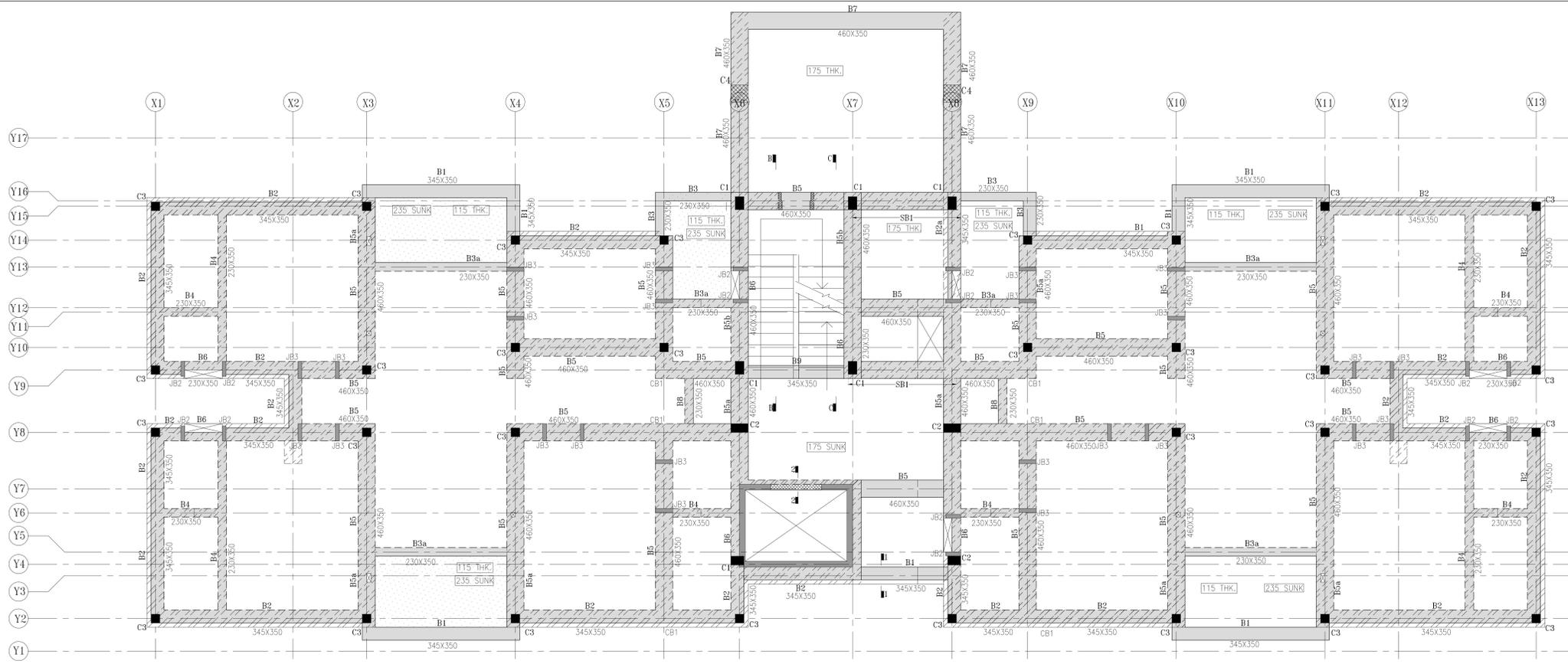
FIRST FLOOR SLAB PLAN AT +3.300M LVL(F.F.L.)
