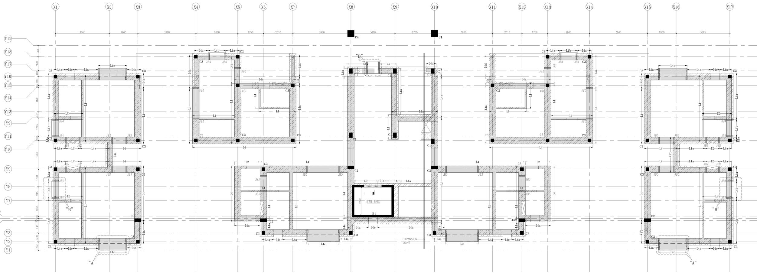
TYPICAL FLOOR LINTEL PLAN AT +5.400/8.700/12.00M LVL (F.F.L.)
