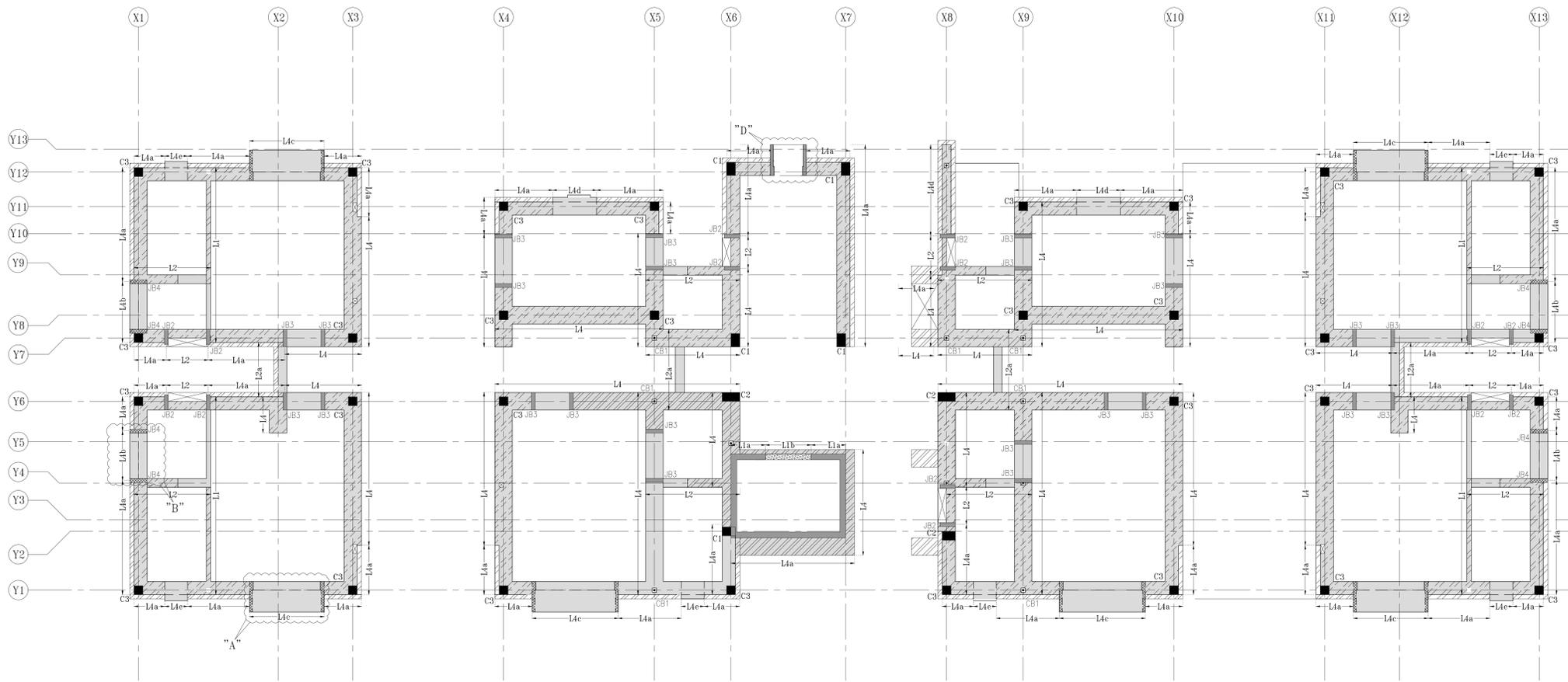
TYPICAL FLOOR LINTEL PLAN AT +5.400/+8.700/+12.00M LVL.
