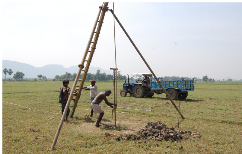
Soil testing being carried out at the Nalanda University construction Site
