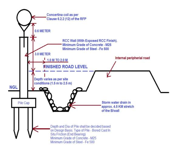
The entire wall shall have exposed RCC finish except the external surface of the 2.5 Km stretch adjacent to SH 71 shall be veneered with decorative Rajasthan Sand Stones with requisite thickness and colour. Design/pattern shall be approved by the Engineer-In-Charge.
