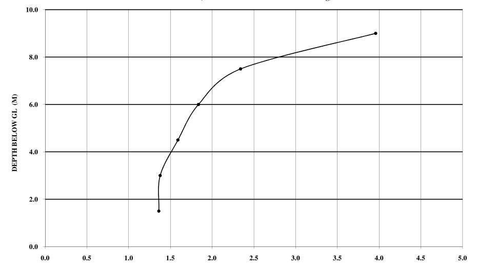
FACTOR OF SAFETY (I.E. RATIO OF LIQUFACTION RESISTANCES OF THE SUB SOIL STRATA TO SHEAR STRESS INDUCES DUE TO EARTHQUAKE )
